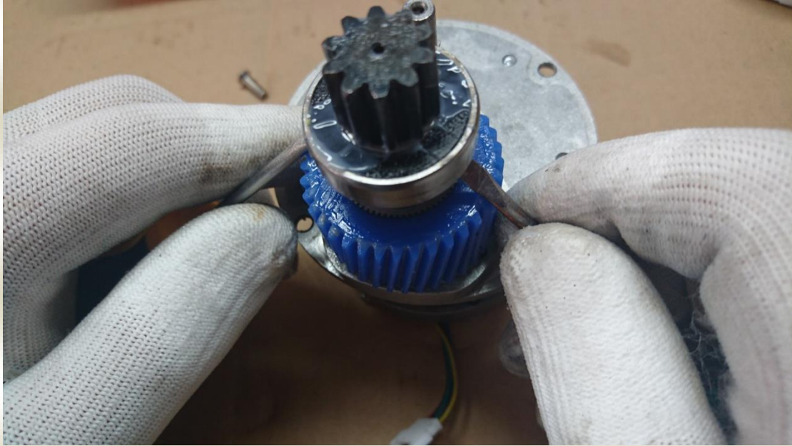
取下尼龙齿轮组件 take off nylon gear assembly
